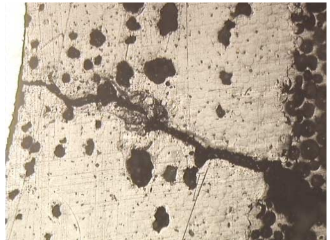
Fig. 4 Crack detection (magnification, 100x)
