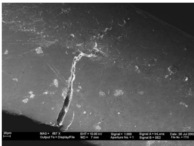
Fig. 2 View under the scanning electron microscope of a sample from section 1 (vacuum mixed cement, stem size 5, 657x magnification). A 150 \mu\text{m} crack beginning in the area between the prosthesis and the bone cement is seen
